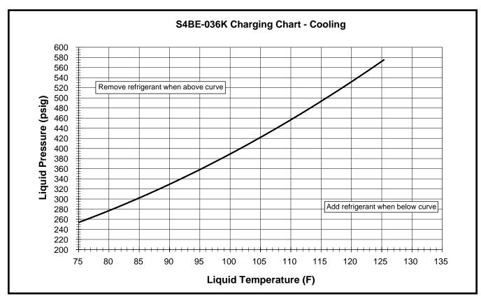
Figure 6. Charging Chart for S4BE-036 Series (3 Ton Units) - TXV Matches
