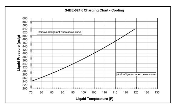
Figure 4. Charging Chart for S4BE-024 Series (2 Ton Units) - TXV Matches
