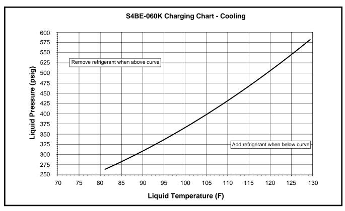
Figure 9. Charging Chart for S4BE-060 Series (5 Ton Units) - TXV Matches
