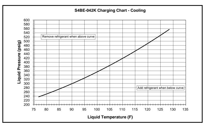
Figure 7. Charging Chart for S4BE-042 Series (3.5 Ton Units) - TXV Matches
