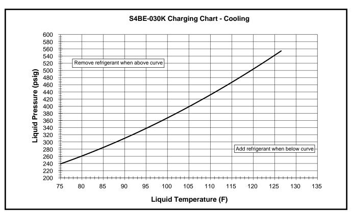
Figure 5. Charging Chart for S4BE-030 Series (2.5 Ton Units) - TXV Matches
