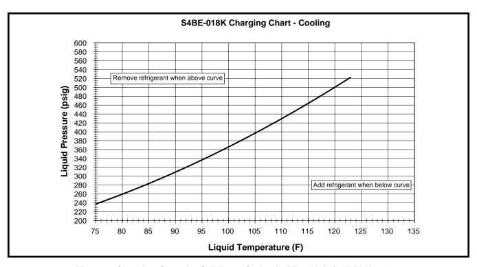
Figure 3. Charging Chart for S4BE-018 Series (1.5 Ton Units) - TXV Matches
