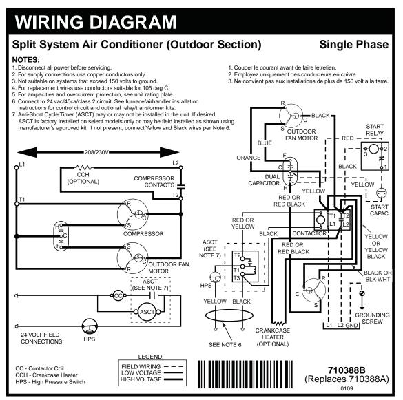
Figure 10. Wiring Diagram for S4BE Single Phase Models (without Comfort Alert)
