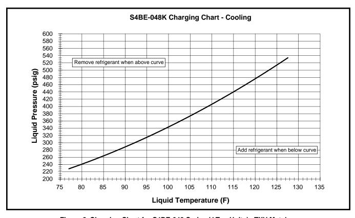
Figure 8. Charging Chart for S4BE-048 Series (4 Ton Units) - TXV Matches
