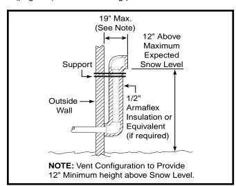
Figure 9. Alternate Horizontal Vent Installation
