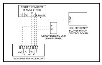
Figure 22. Wiring Configuration 1
