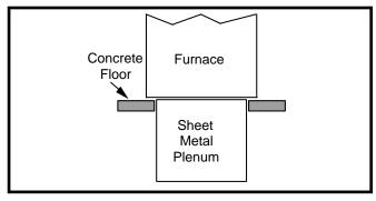
Figure 13. Furnace on a Concrete Slab
