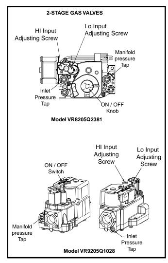
Figure 27. HI & LO Input Adjusting Screws
