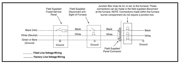
Figure 21. Line Voltage Field Wiring
