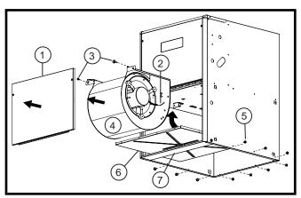
Figure 18. Bottom Panel Removal
