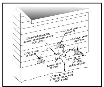
Figure 7. Inlet & Exhaust Pipe Clearances
