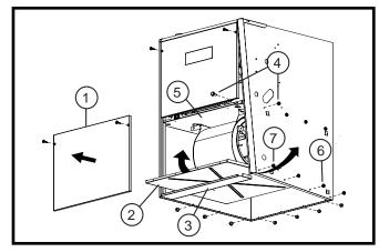
Figure 19. Alternate Removal Method
