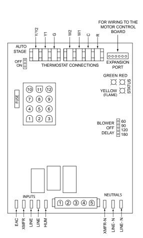
Figure 31. Two-Stage Furnace Control Board
