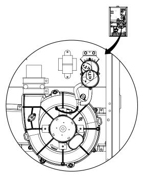
Figure 15. Pressure Switch Tubing for \*TL Downflow Furnaces
