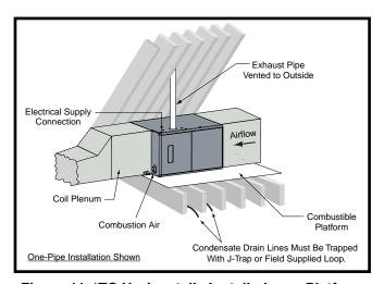
Figure 11. \*TC Horizontally Installed on a Platform
