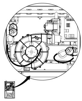
Figure 14. Pressure Switch Tubing for \*TC Upflow / Horizontal Furnaces
