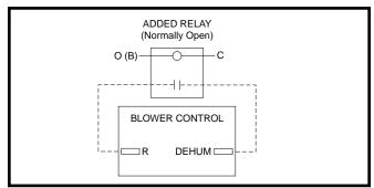
Figure 26. DEHUM Wiring Configuration without Humidistat
