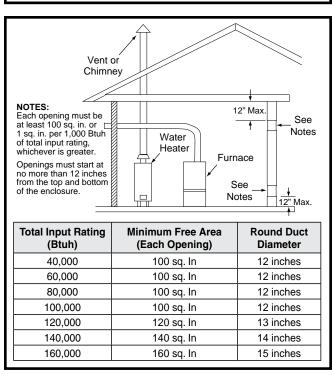
Figure 2. Combustion Air Drawn from Inside
