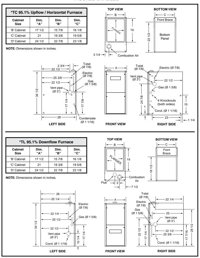
Figure 28. Furnace Dimensions
