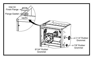
Figure 16. Finish Flange & Rubber Grommets
