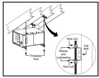
Figure 12. \*TC Horizontally Suspended in an Attic
