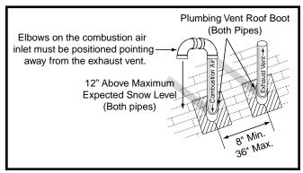
Figure 10. Vertical Vent Termination
