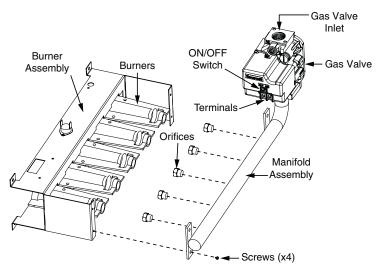
Figure 1. Burner & Manifold Assembly
