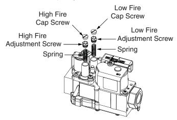
Figure 5. Pressure Regulator Spring & Adjustment Screw Removal
