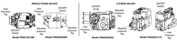
Figure 6. Inlet & Manifold Pressure Tap Locations
