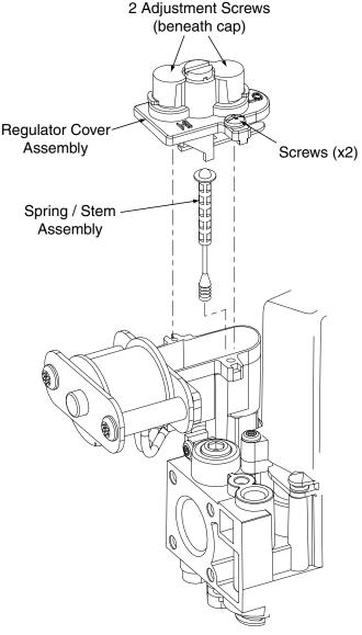
Figure 4. Spring / Stem Assembly Removal
