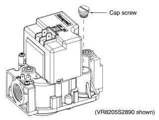
Figure 2. Cap Screw Removal
