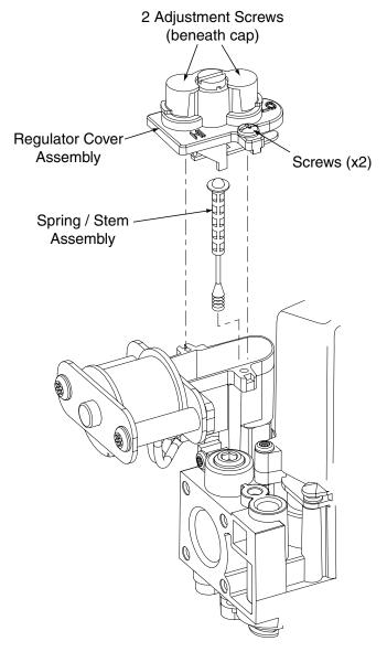
Figure 4. Spring / Stem Assembly Removal
