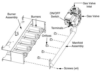
Figure 1. Burner & Manifold Assembly
