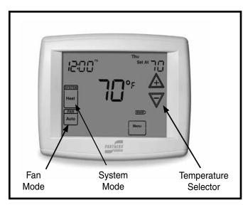
**Figure 1. Typical Digital Thermostat**
