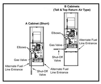
Figure 18. Typical Gas Connections
