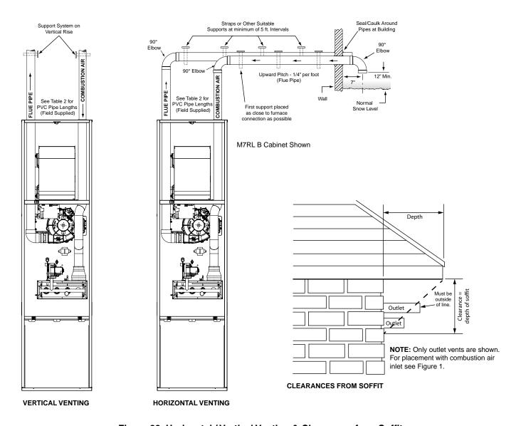
Figure 28. Horizontal / Vertical Venting & Clearances from Soffit
