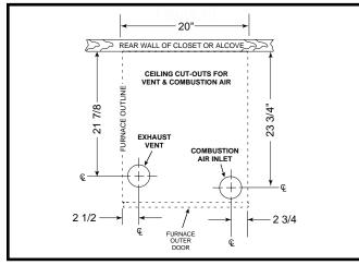
Figure 10. Ceiling Cut-Out Dimensions
