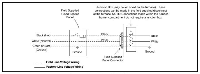
Figure 21. Line Voltage Field Wiring
