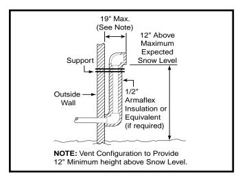
Figure 3. Alternate Horizontal Vent Installation
