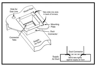
Figure 11. Finger Tabbed Duct Connector
