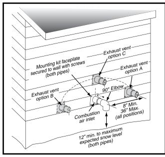
Figure 1. Inlet & Exhaust Pipe Clearances
