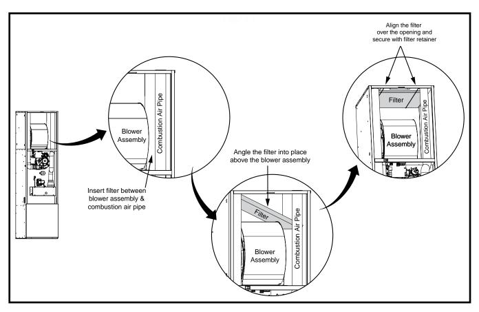
Figure 7. Filter Installation
