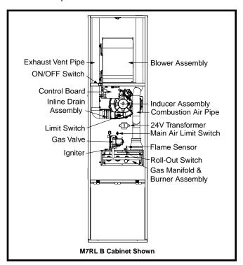
Figure 23. Furnace Components
