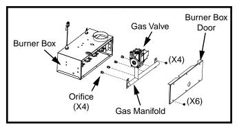
Figure 20. Orifice Removal
