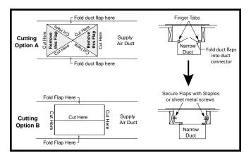
Figure 12. Narrow Air Ducts - Option 1
