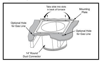
Figure 15. Round Duct Connector
