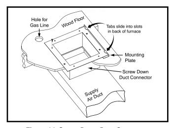
Figure 14. Screw-Down Duct Connector
