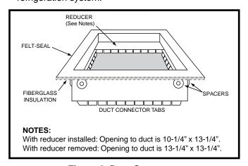
Figure 8. Duct Connector
