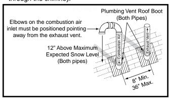
Figure 4. Vertical Vent Termination
