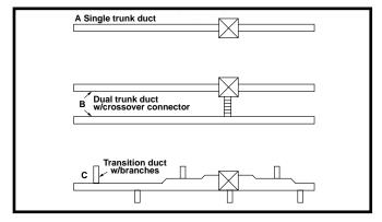
Figure 6. Typical Supply Duct Systems
