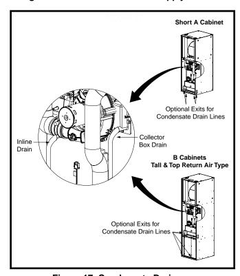
Figure 17. Condensate Drainage
