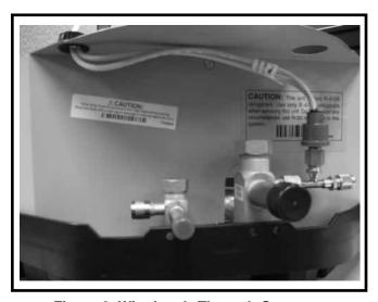
Figure 2. Wire Leads Through Grommet
