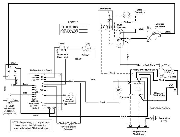
Figure 3. Field Wiring Diagram for Mild Weather Control Kit (Heat Pump with Condensor Fan Motors Up to 5 Amps)
