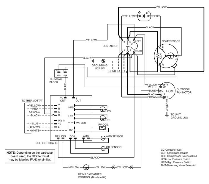
Figure 4. Field Wiring Diagram for Mild Weather Control Kit (Heat Pump with ECM Outdoor Fan Motor - 14 SEER Units)
