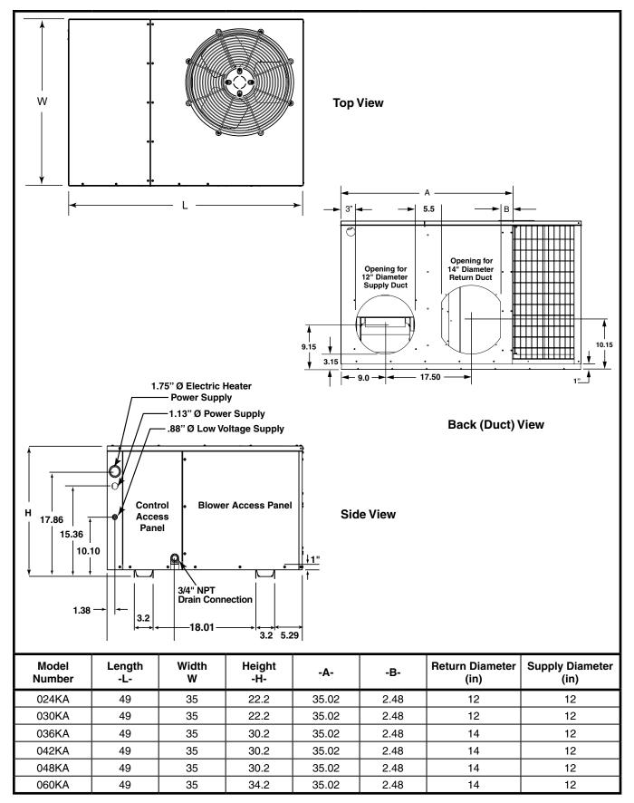
Figure 9. Physical Data & Unit Dimensions
