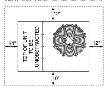
Figure 1. Minimum Unit Clearances
