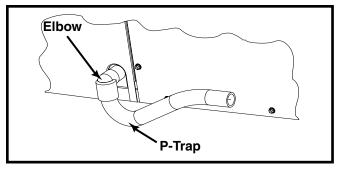
Figure 6. Drain Trap
