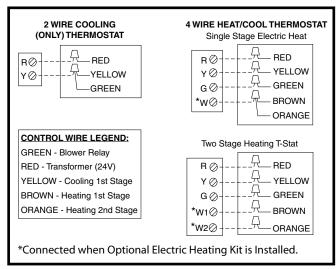
**Figure 8. Low Voltage Connections**
