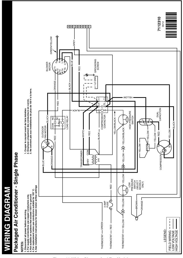
Figure 11. Wiring Diagram for 3 Ton Models
