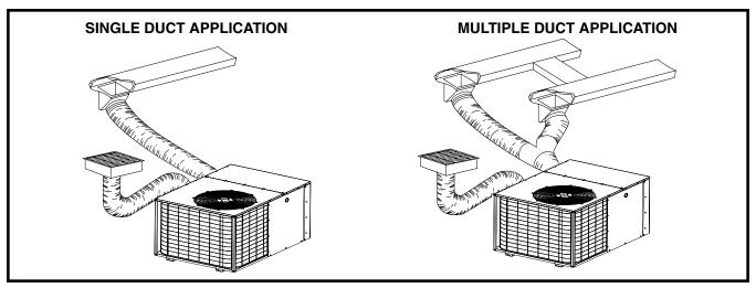
Figure 2. Single & Multiple Duct Applications
