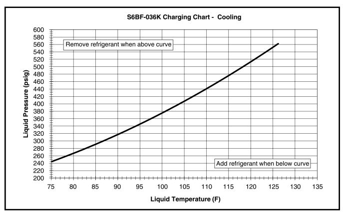
Figure 4. Charging Chart for 3 Ton Units S6BF-036 Series (TXV Matches)
