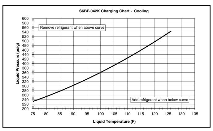
Figure 5. Charging Chart for 3.5 Ton Units S6BF-042 Series (TXV Matches)
