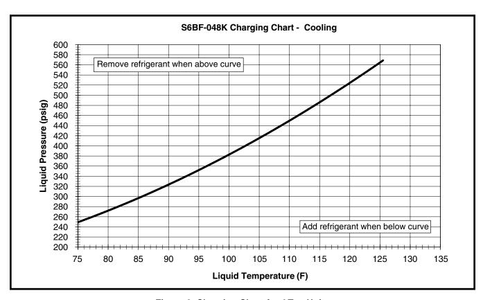
Figure 6. Charging Chart for 4 Ton Units S6BF-048 Series (TXV Matches)
