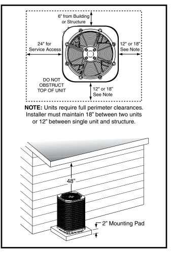
Figure 1. Clearance Requirements
