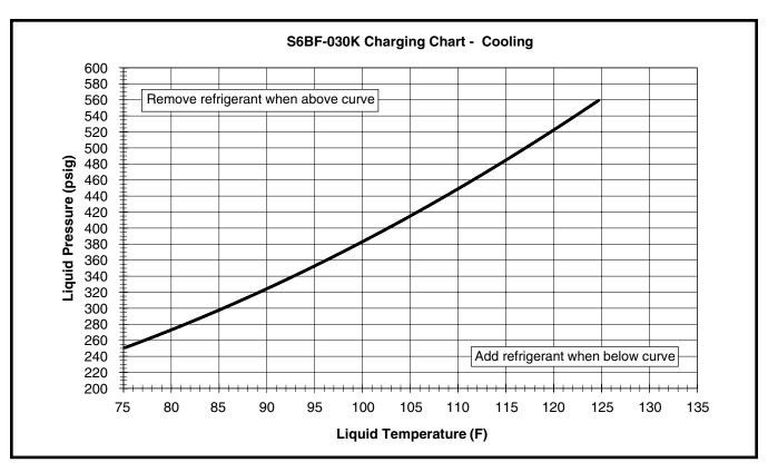
Figure 3. Charging Chart for 2.5 Ton Units S6BF-030 Series (TXV Matches)
