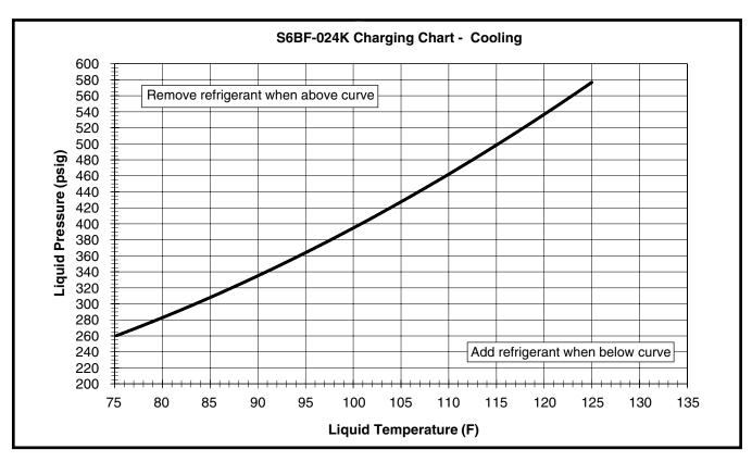
Figure 2. Charging Chart for 2 Ton Units S6BF-024K Series (TXV Matches)
