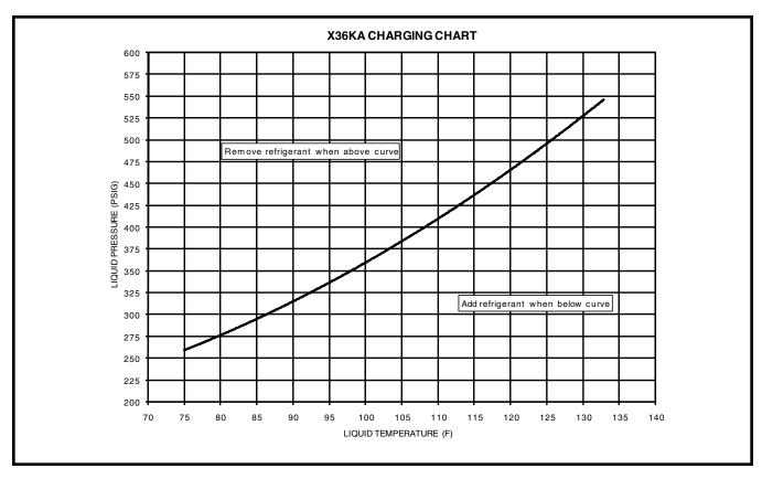
Figure 10. Charging Chart for 3 Ton Units
