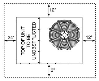
Figure 1. Minimum Unit Clearances
