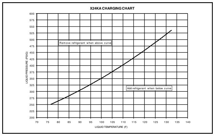
Figure 9. Charging Chart for 2 Ton Units
