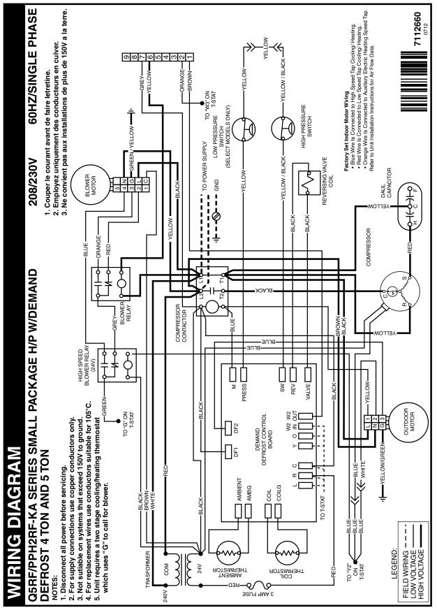
Figure 14. Wiring Diagram - 4 & 5 Ton Units
