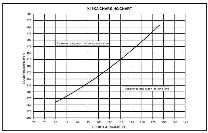
Figure 11. Charging Chart for 4 Ton Units
