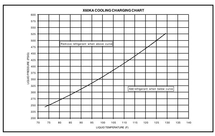
Figure 12. Charging Chart for 5 Ton Units
