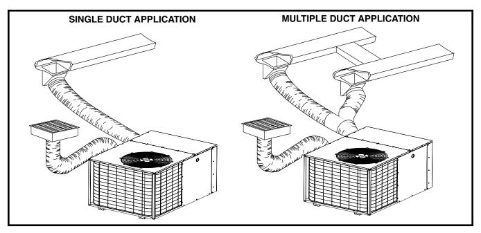
**Figure 3. Typical Duct Applications**
