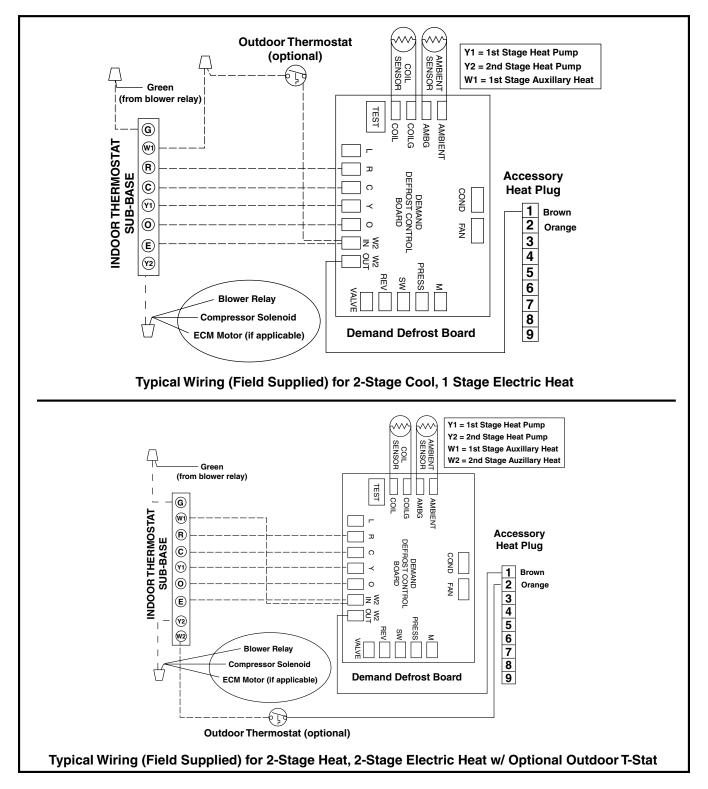
Figure 7. Typical Heat Pump Thermostat Connections
