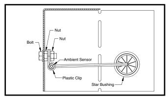
**Figure 6. Ambient Sensor Mounting**
