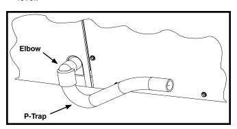
Figure 4. Drain Trap
