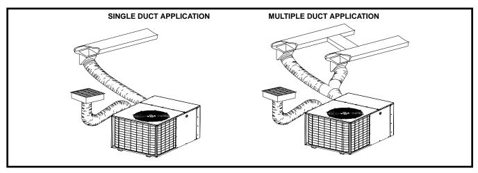
Figure 2. Single & Multiple Duct Applications
