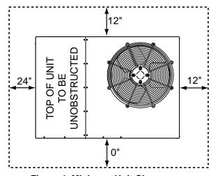
Figure 1. Minimum Unit Clearances
