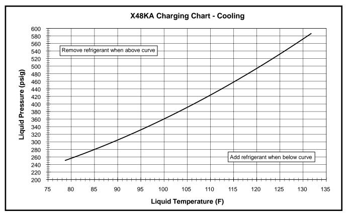
Figure 10. Charging Chart for 4 ton Units
