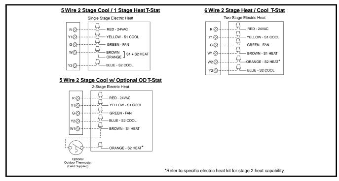
Figure 6. Typical Wiring (Field Supplied) for 2-Stage Cool & 1 or 2-Stage Electric Heat
