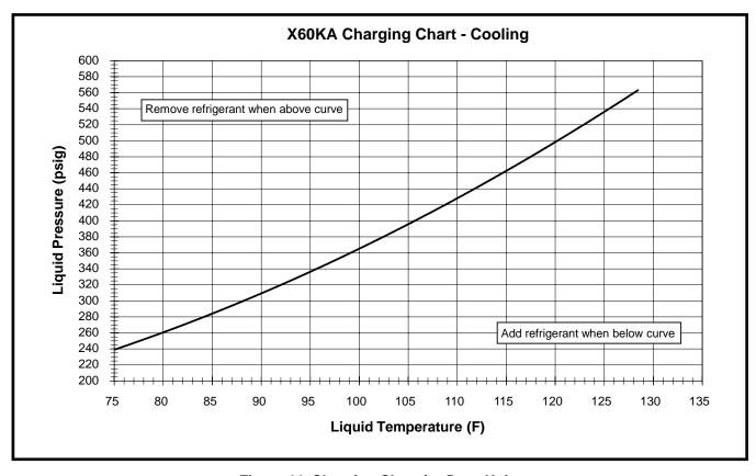
Figure 11. Charging Chart for 5 ton Units
