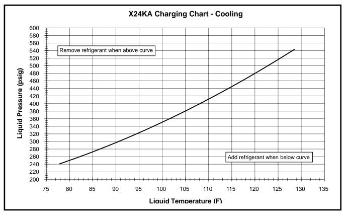
Figure 8. Charging Chart for 2 ton Units
