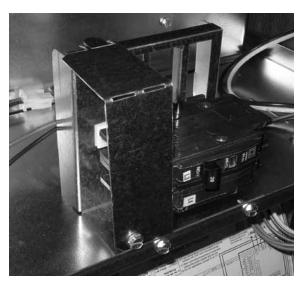
Figure 5. Line Cover Installed
