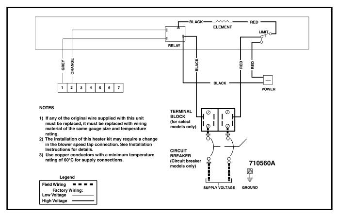
Figure 7. Wiring Diagram for H6HK Single Stage Air Handler with Circuit Breaker(s) - 5 kw Series
