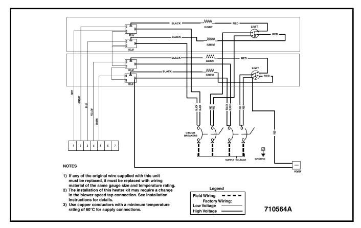
Figure 10. Wiring Diagram for H6HK Single Stage Air Handler with Circuit Breaker(s) - 20 kw Series
