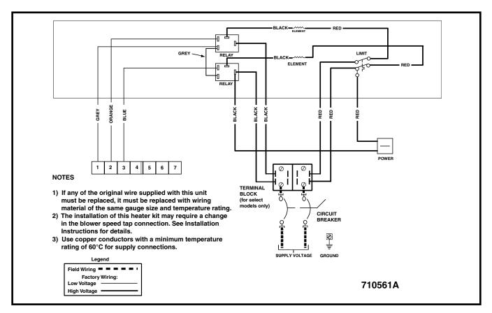
Figure 8. Wiring Diagram for H6HK Single Stage Air Handler with Circuit Breaker(s) - 8/10 kw Series
