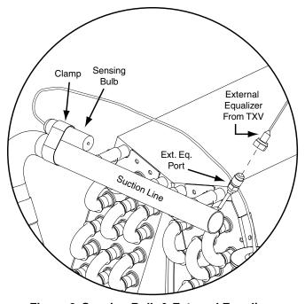
Figure 6. Sensing Bulb & External Equalizer
