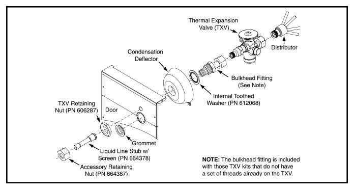
Figure 5. TXV Assembly As Installed
