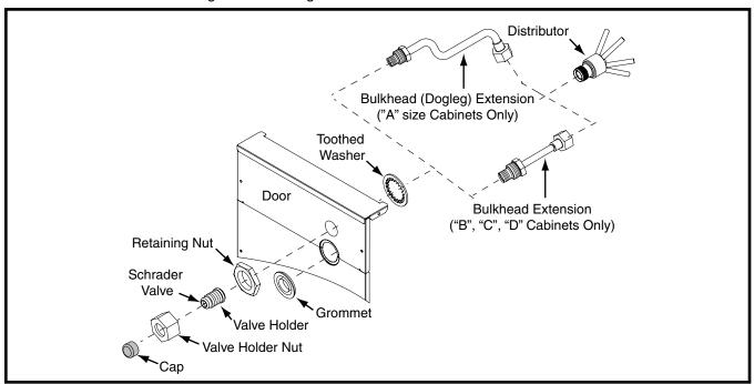
Figure 4. C6 Coil Assembly As Shipped
