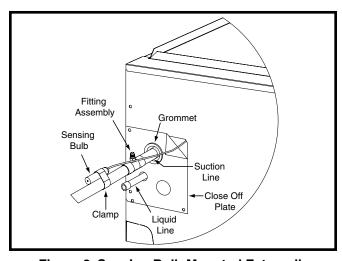
Figure 3. Sensing Bulb Mounted Externally
