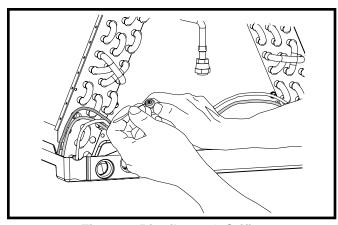
Figure 1. Distributor & Orifice
