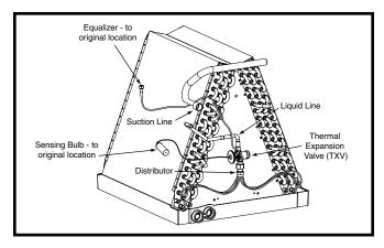
Figure 2. C5 Coil With TXV Installed
