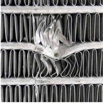
Figure 3. Damaged Micro-Channel Example
