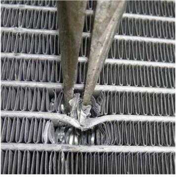
Figure 4. Micro-Channel Damage Removal
