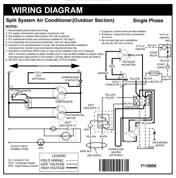
Figure 9. S6BD Wiring Diagram (1.5 - 2.5 Ton Units)
