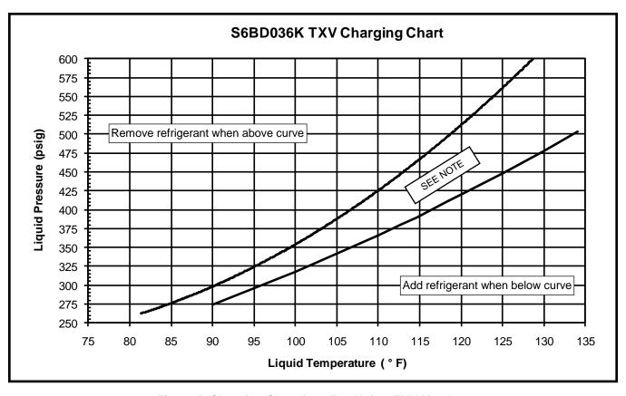
Figure 5. Charging Chart for 3 Ton Units - TXV Matches
