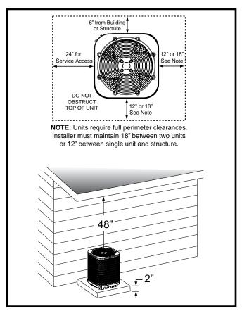
Figure 1. Clearance Requirements
