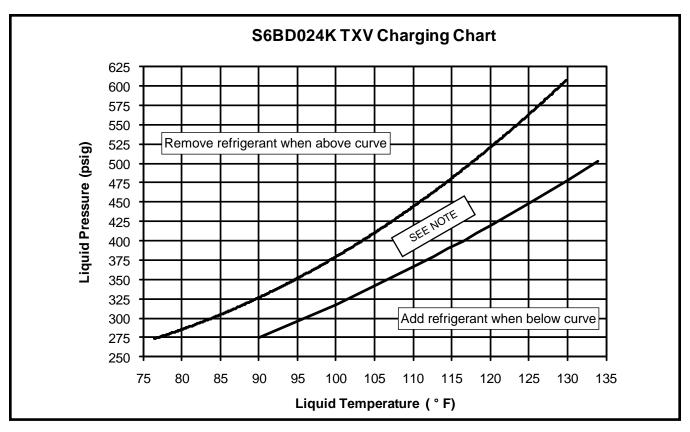
Figure 3. Charging Chart for 2 Ton Units - TXV Matches
