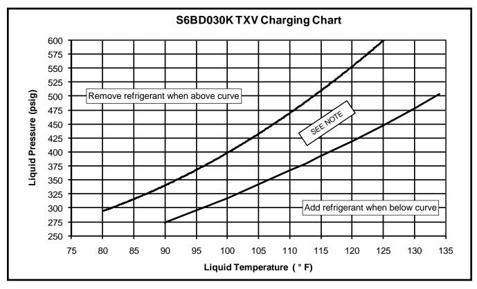
Figure 4. Charging Chart for 2.5 Ton Units - TXV Matches
