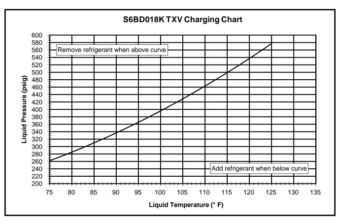
Figure 2. Charging Chart for 1.5 Ton Units - TXV Matches
