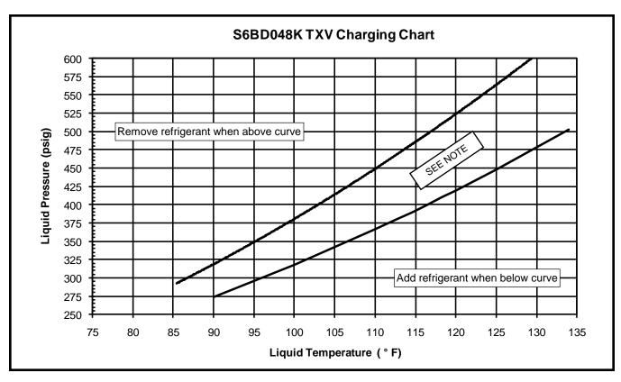
Figure 7. Charging Chart for 4 Ton Units - TXV Matches
