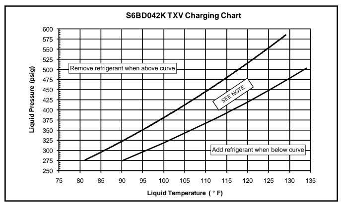
Figure 6. Charging Chart for 3.5 Ton Units - TXV Matches
