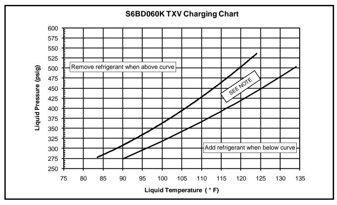
Figure 8. Charging Chart for 5 Ton Units - TXV Matches
