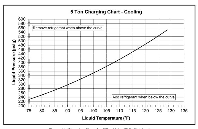
Figure 11. Charging Chart for 5 Ton Units (TXV Matches)
