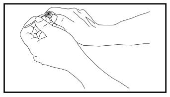
Figure 3. Removal of Orifice
