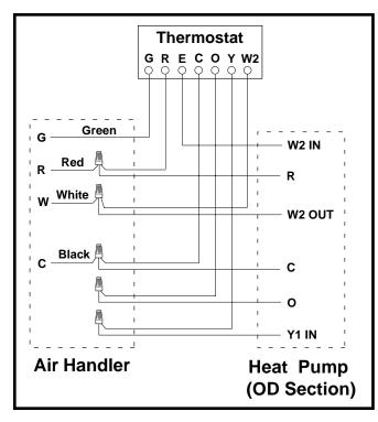
**Figure 4. Typical Thermostat Connections**
