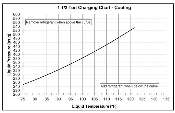
Figure 5. Charging Chart for 1.5 Ton Units (TXV Matches)
