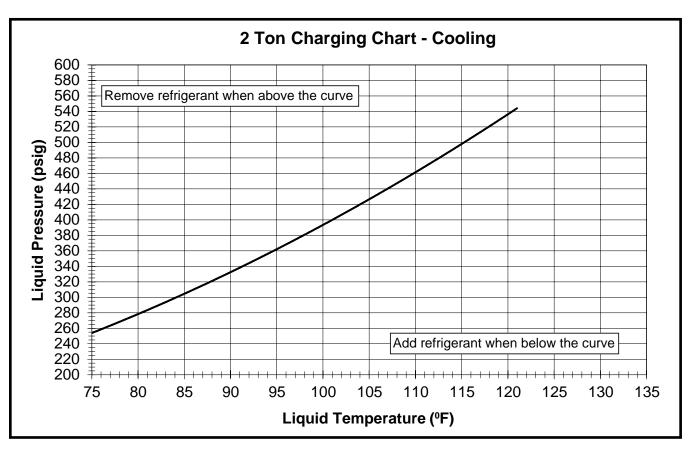
Figure 6. Charging Chart for 2 Ton Units (TXV Matches)
