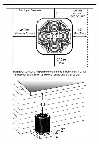
Figure 1. Clearance Requirements
