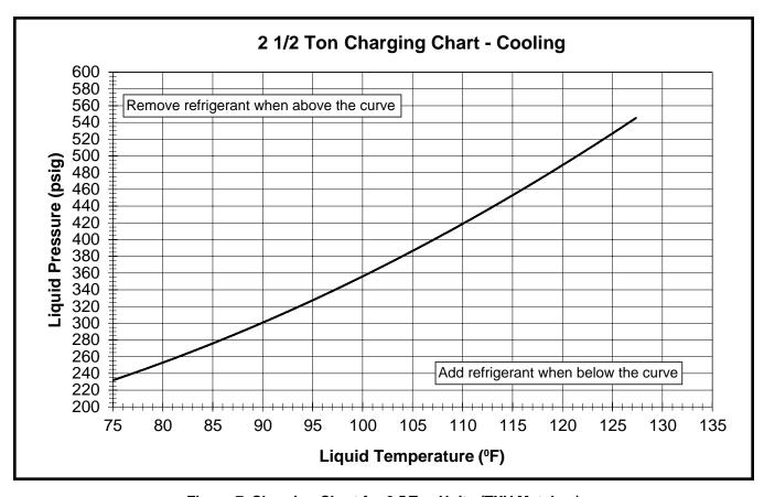
Figure 7. Charging Chart for 2.5 Ton Units (TXV Matches)
