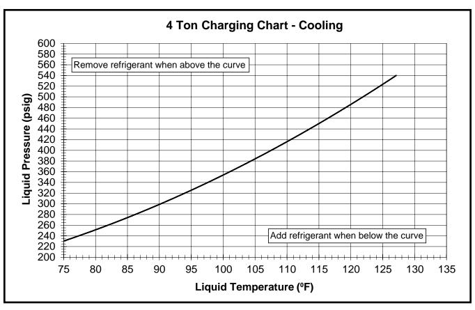
Figure 10. Charging Chart for 4 Ton Units (TXV Matches)
