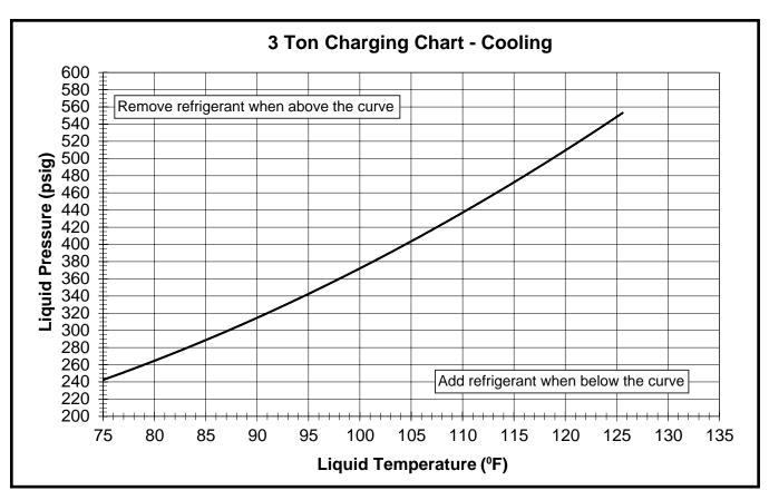
Figure 8. Charging Chart for 3 Ton Units (TXV Matches)
