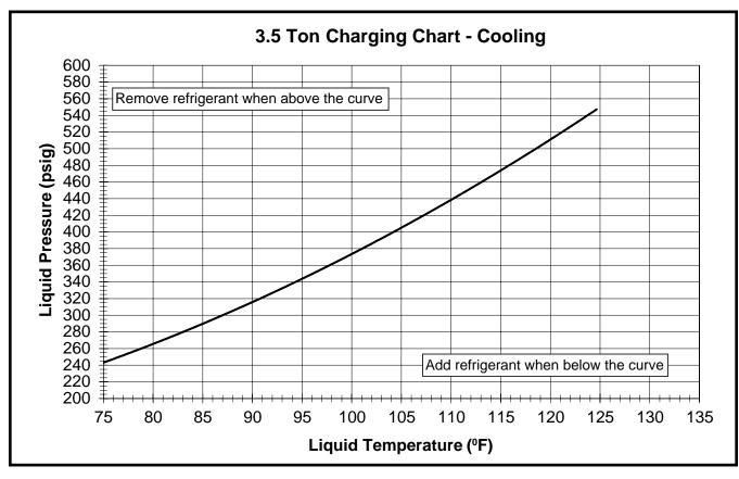
Figure 9. Charging Chart for 3.5 Ton Units (TXV Matches)
