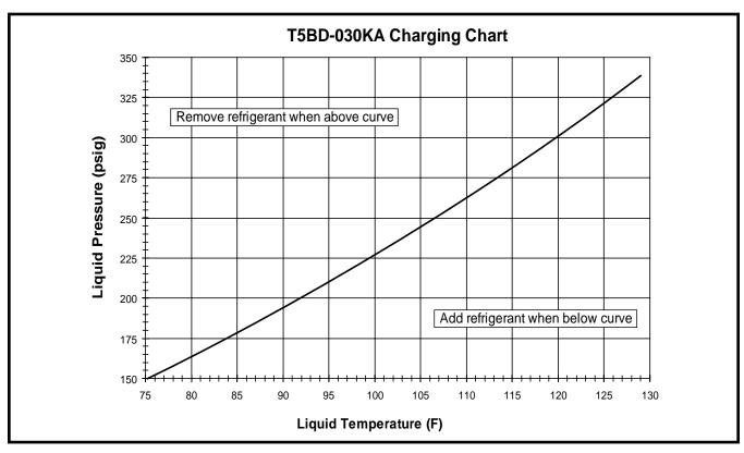
Figure 7. Charging Chart for 2.5 Ton Units
