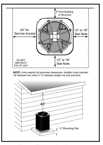
Figure 2. Clearance Requirements
