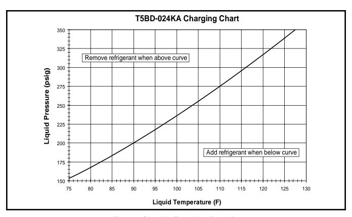
Figure 6. Charging Chart for 2 Ton Units
