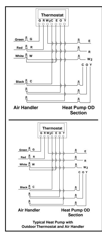
**Figure 3. Typical Thermostat Connections**
