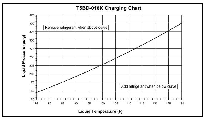
Figure 5. Charging Chart for 1.5 Ton Units
