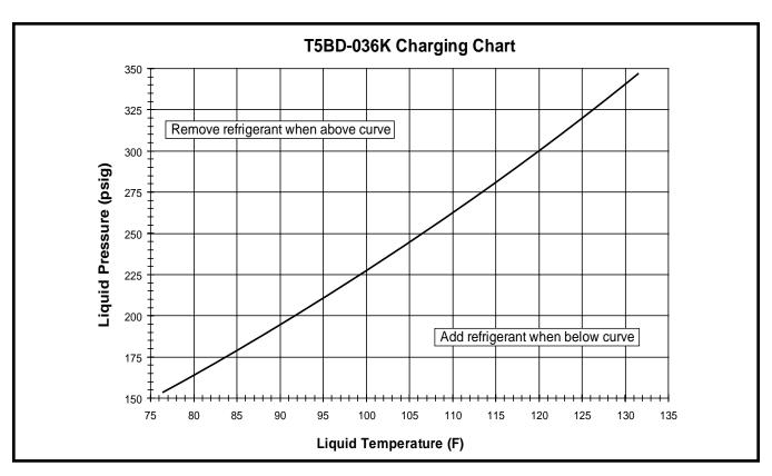
Figure 8. Charging Chart for 3 Ton Units
