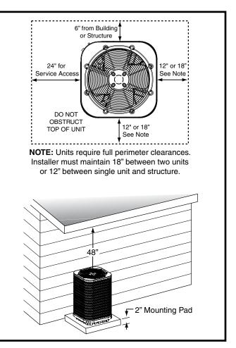
Figure 1. Clearance Requirements
