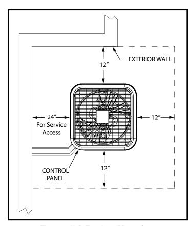
Figure 1. Unit Envelope Dimensions
