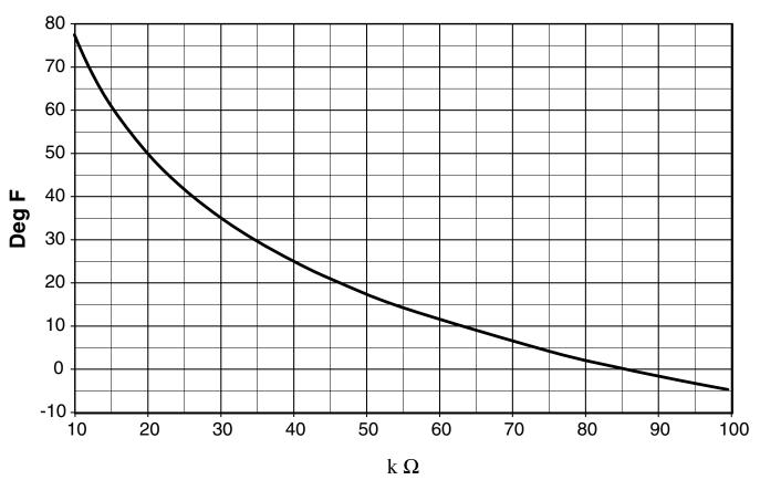
**Figure 10. Temperature Sensor Resistance Charts**
