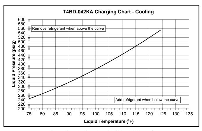
Figure 6. Charging Chart for 3.5 Ton Units (TXV Matches)
