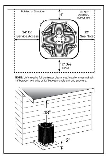
Figure 1. Clearance Requirements
