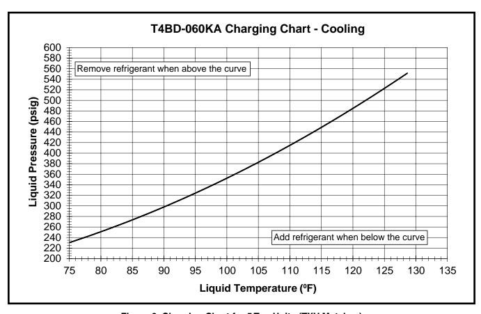
Figure 8. Charging Chart for 5 Ton Units (TXV Matches)
