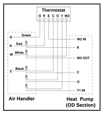
Figure 4. Typical Thermostat Connections
