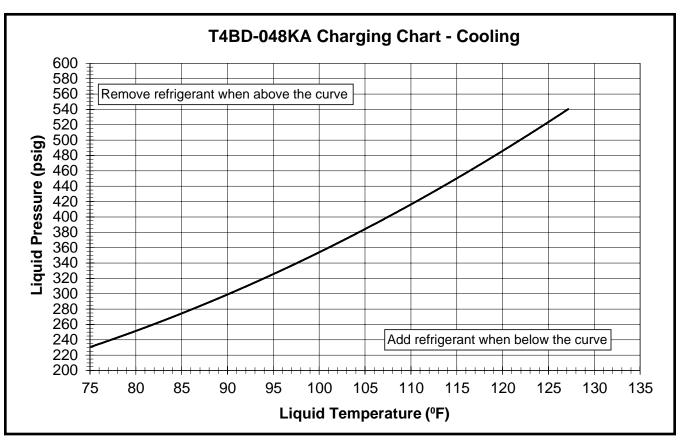
Figure 7. Charging Chart for 4 Ton Units (TXV Matches)
