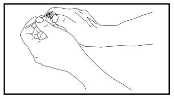
Figure 3. Removal of Orifice
