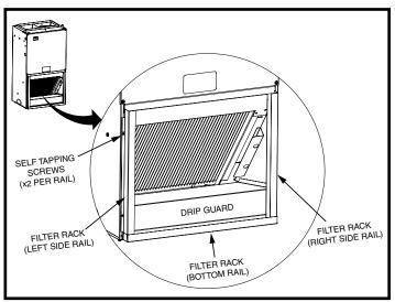
Figure 2. Drip Guard Installed
