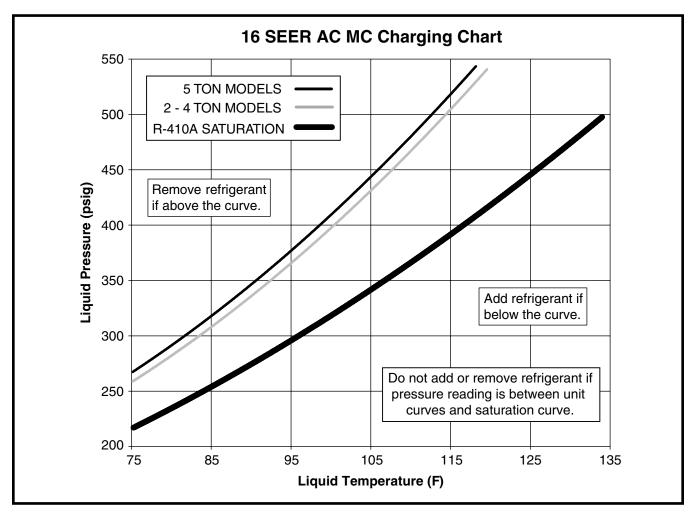
Figure 4. Charging Chart for 2-5 Ton Models
