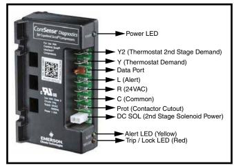
Figure 2. CoreSense™ Diagnostics Module
