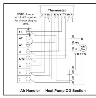
Figure 2. Typical 2 - Stage Heat Pump w/ Optional Outdoor Thermostat and Variable Speed Air Handler
