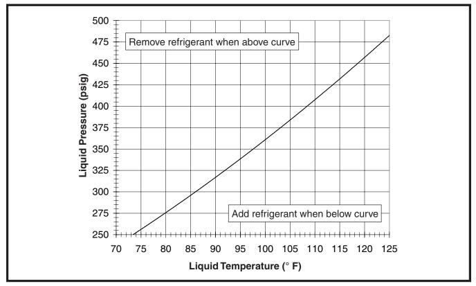
Figure 5. Charging Chart for 3 Ton Units
