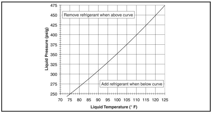
Figure 4. Charging Chart for 2 Ton Units
