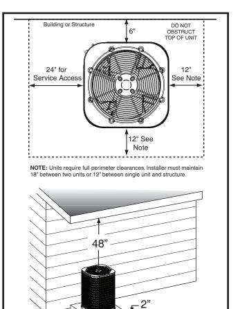
Figure 1. Clearance Requirements
