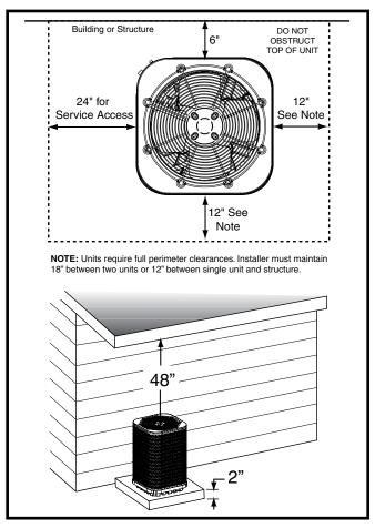
**Figure 1. Clearance Requirements**
