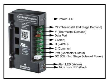
Figure 3. CoreSense™ Diagnostics Module
