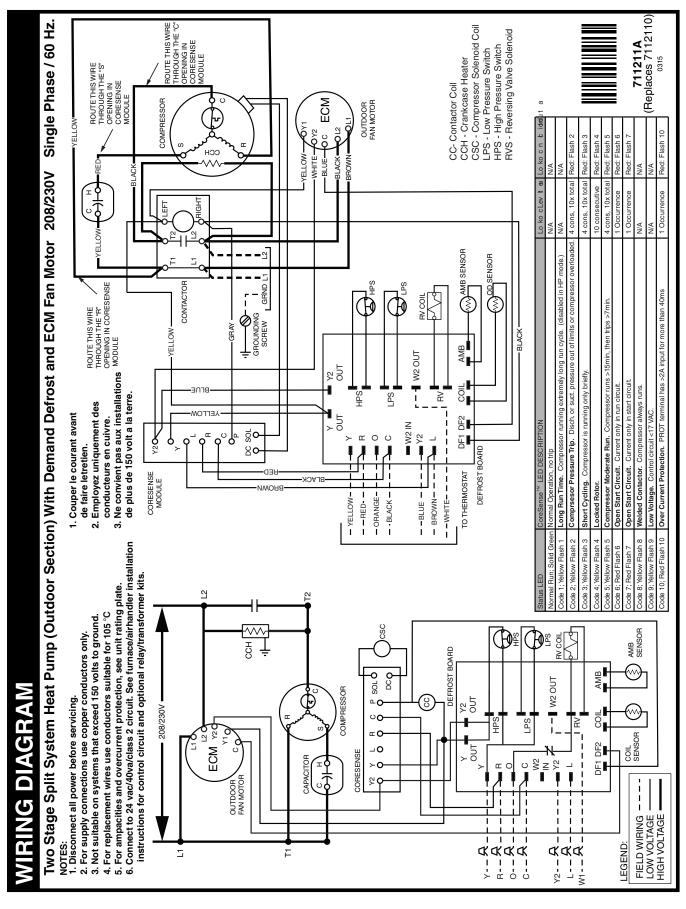
Figure 14. W.D. for 4 & 5 Ton Models With CoreSense™
