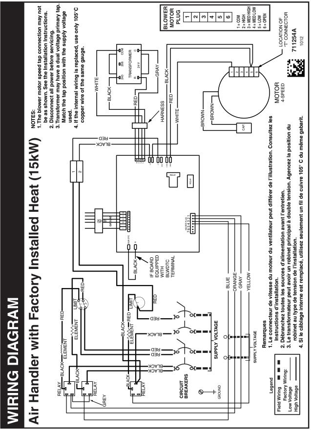
Figure 14. B6BV Air Handler Equipped With PSC Motor & 15 kw Heater Kit (B Size Cabinet Only)
