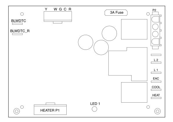
Figure 10. Single Stage Control Board
