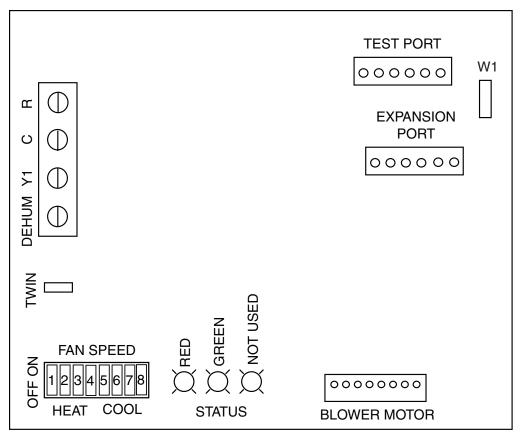
Figure 12. Two-Stage Fixed Speed Motor Control Board
