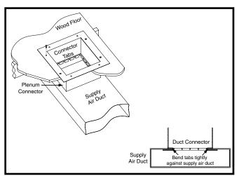
Figure 5. Duct Connector Installed
