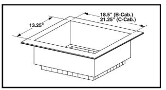
Figure 3. Plenum Adapter
