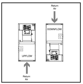
Figure 2. Installation Configurations
