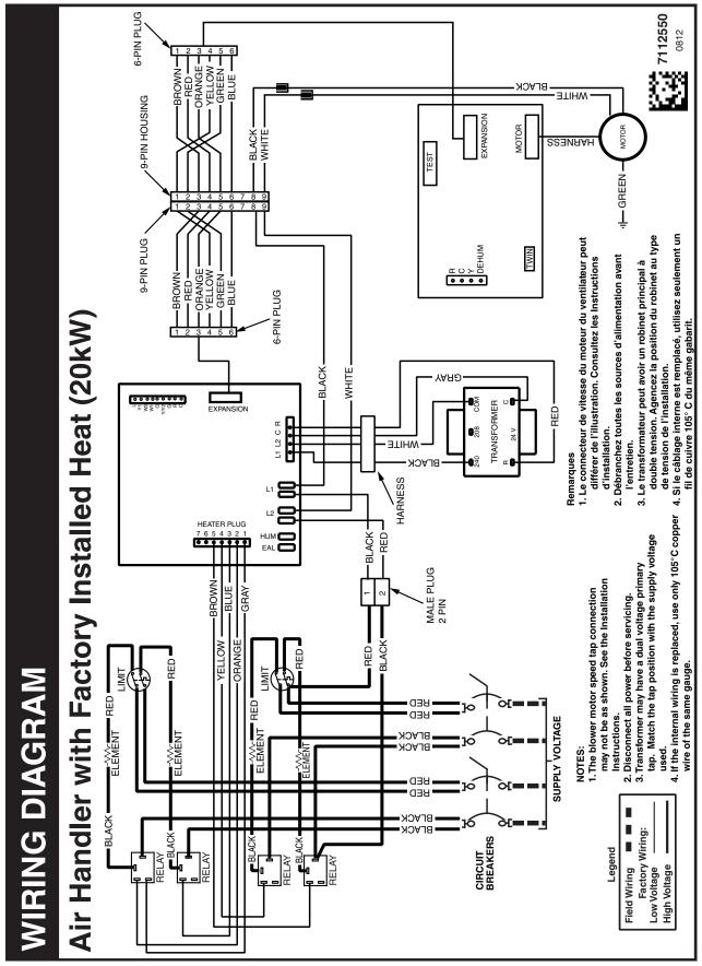
Figure 16. B6BV Air Handler Equipped With FSHE Motor & 20 kw Heater Kit (C Size Cabinet Only)
