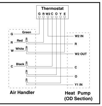
Figure 2. Typical Thermostat Connections
