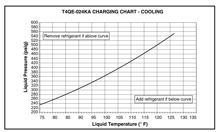
Figure 4. Charging Chart for 2.5 Ton Models (TXV Matches)
