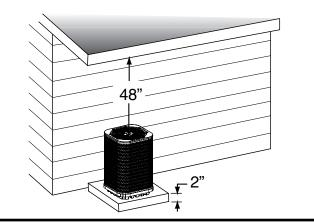
Figure 1. Clearance Requirements
