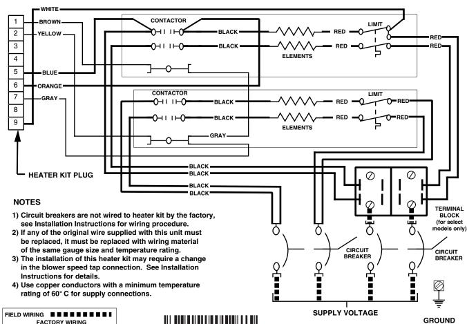
20 kW, 240 VAC, 1-Phase Electric Heater Kit
