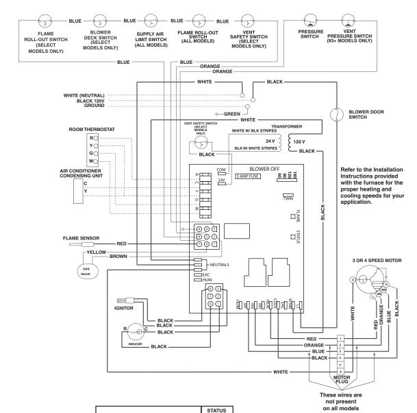
RFD **FAULT CONDITION** LIGHT Power On 1 FLASH Limit Circuit Open or External Load On "W' Pressure Switch is Open with Inducer On 2 FLASHES Pressure Switch is Closed with Inducer Off 3 FLASHES Ignition Failure (Check Ground) 4 FLASHES 115 VAC & Neutral Reversed or no Ground 5 FLASHES False Flame or Gas Valve Relay Shorted Continuous Power Off OFF FLAME YELLOW LIGHT **FAULT CONDITION** Low Flame Sensor Signal Continuous Flash Flame Present ON
