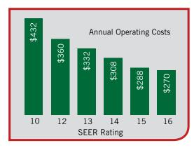
Annual costs based on 36,000 Btu unit, 1500 cooling load hours, and .08/kwh. Actual costs may vary depending on climate conditions, energy rates and patterns of usage.
