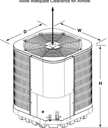
Air Discharge Allow Adequate Clearance for Airflow
