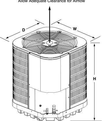
Air Discharge Allow Adequate Clearance for Airflow
