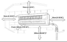
\*A mounting height of 98-5/8" from the floor is recommended, however, this height may not be available for installations with lower ceilings. In these cases, the unit should be placed as high on the wall as possible, while maintaining a ceiling clearance of 5-15/16" or greater
