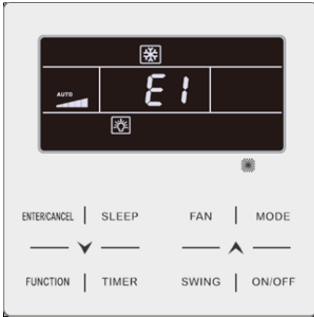
Fig.5.1 Display of Outdoor Unit High Pressure Protection
